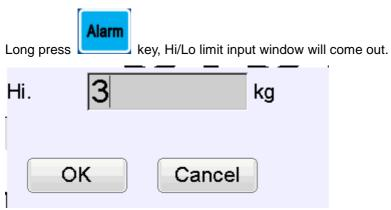
Press number keys to input high limit. Please take attention on the right unit show area. After input, press [OK], the Low limit window will pop-up. Use number keys to input low limit, then press [OK]. Note: The low limit value must lower than high limit value.
